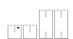
2. Insert the dowels in the half-H boards holes.
