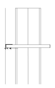
**3.** There is no need to drill in the board as the top parts of the brackets are locking the shelf.
