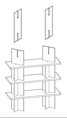
**10.** Insert the dowels and slide the last horizontal board.
