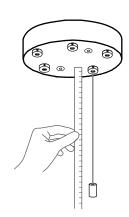
Determine the overall drop for the pendant fixture.
