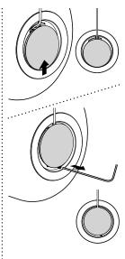
Slide the cap so the two circles are concentric. Partially unthread the exposed screw to lock the cap in position. DO NOT unthread the screw all the way.
