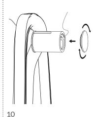
Screw frame cap back onto the frame
