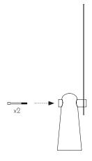
**3.** Set the cover and lock it with the small screw under the cylinder.
