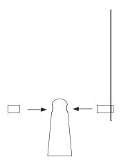
**2.** Holding the mirror, insert the two big screws at the back of the mirror and screw alternately until the mirror is locked.
