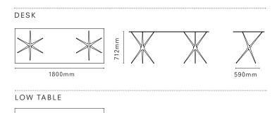
The Supernova is a completely dynamic, self-levelling desk trestle, cast entirely from recycled aluminium with a toughened glass top. Exceptionally simple to orientate, the star shaped structure is able to be positioned freely to create a dynamic sculptural shape, vertically for the desk or horizontally for the low table.
